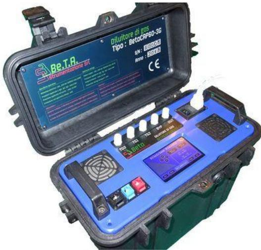
The diluter uses 60 equal capillaries and a solenoid valves network that directs to each capillary the first gas to be diluted, the second or the diluting gas.
