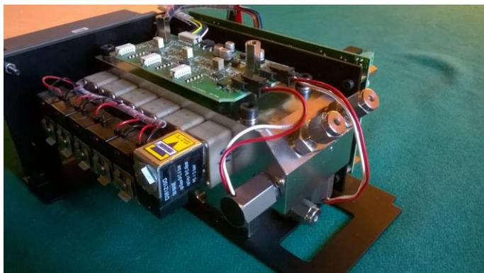
Finally, to ensure uniformity of capillaries temperature, these are "embedded" between the two shells of solid material (fluorinated resin or stainless steel). The best performances are got immediately after the switching on and are maintained for years.
